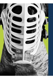
While the device can operate correctly without the placement of a counterweight in the front, its use is recommended to reduce the chances of damage to the fruit trees. The counterweight is placed in the perforation of the front flap, and a through screw with washers and nuts should be used in sufficient quantity to reach the necessary weight.
